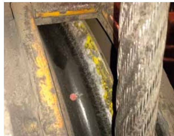
If the red dot is still present, the sheave is still within the technical tolerances as designed by the maker.
